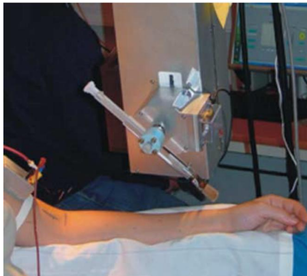
Figure 11. A rotary machine will be used to deliver a controlled stroking of the stimulus in order to measure the hedonic ratings in the various groups of participants. Reprinted from “Discriminative Touch and Emotional Touch,” by F. M. et al., 2007, Canadian Journal of Experimental Psychology , 61(3), 173-183.
