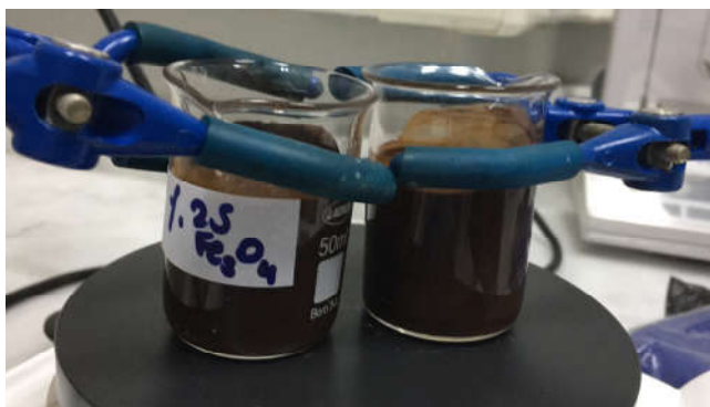
Figure 1. 20% and 25% \text{Fe}_3\text{O}_4 suspensions on Heidolph MR Hei-Standard magnetic stirrer
