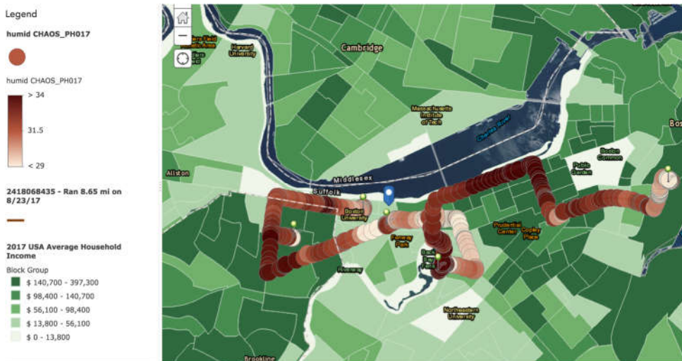
Figure 2. Humidity ArcGIS Map Layer Humidity data collected by the Particle Photon while driving through neighborhoods encompassing a range of average household income.
