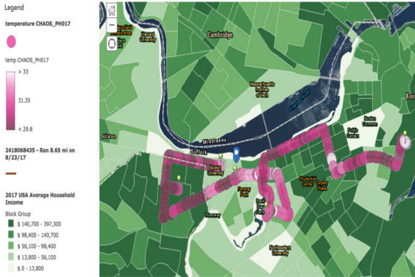
Figure 1. Temperature ArcGIS Map. Temperature data collected by the Particle Photon while driving through neighborhoods encompassing a range of average household income.
