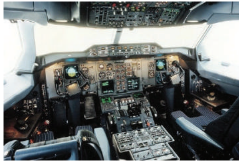
Figure 6. The A300 Cockpit, with a Primary Flight Display in front of each pilot
