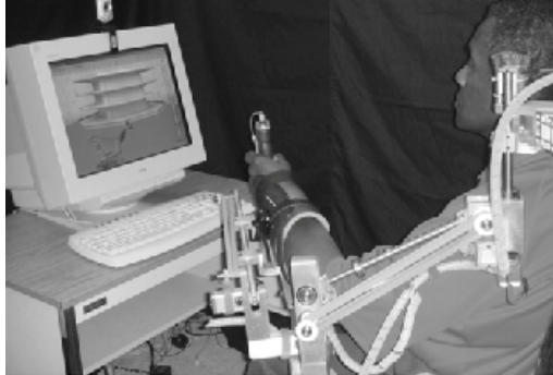
Figure 2. The VR and robotic TREX arm orthosis used by Housman et al 13
