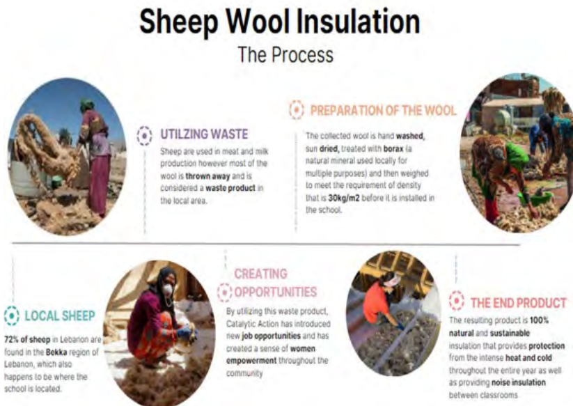
Figure 15. This figure illustrates the process of creating the sheep wool insulation that was used in the construction of the Jarahieh School (source: modified by author based on illustrations provided in “Pavilion Re-Claimed in Lebanon”). It outlines the most important steps and shows various context information as well as the significance of the process.
