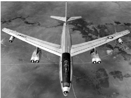
Figure 1. B-47 Stratojet Bomber. This airplane explores the design of swept wing with podded engines, and a fuselage is placed at the centerline of the aircraft. This design is also known as “wing and tube” configuration (Leone, 2019)
