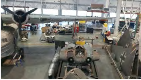
Figure 9. Center-body of Ho 229 Komet Fighter with its removed wings placed on the right in the Smithsonian National Air and Space Museum's Paul E. Garber Restoration Facility in Suitland, Maryland, U.S (Dowling, 2017)
